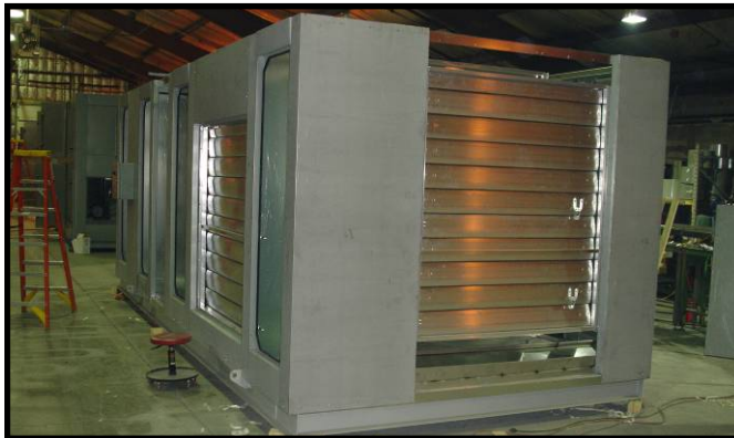
Dampers for exhaust air (left) and supply air (right).
