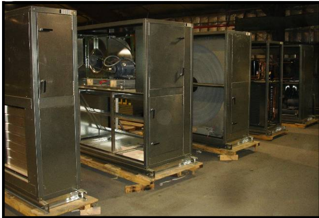
Modular construction with five sections
