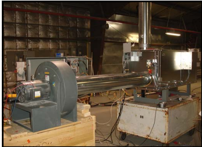
As a part of factory testing, a remote blower was connected to the unit. The precision with which the unit could control the supply air temperature and mass flow rate were verified before it shipped.
