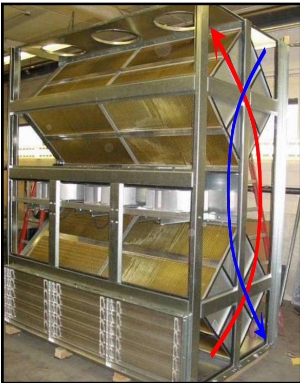
The VFD bolts on to the back side. The double-pass exchanger configuration results in 80% heat transfer effectiveness.
