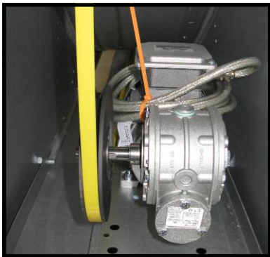
A 1/8 to 1/2 hp gear reduced motor with soft-start requires no maintenance as all components are pre-lubricated and sealed.
