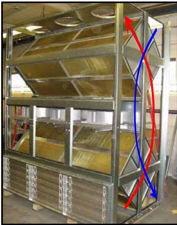
The VFD bolts on to the back side. The double-pass heat exchanger configuration results in 80% heat transfer effectiveness.
