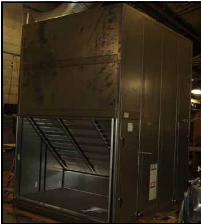
The completed XC Unit with Face-and-Bypass Damper visible through outdoor air opening
